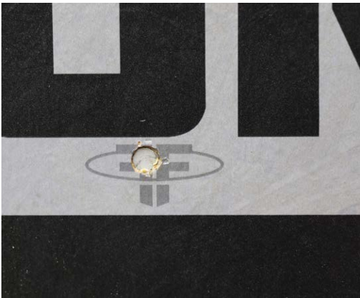
The ForceField system was tested with flush-driven and over-penetrated nails, and passed the water penetration test in both instances.
